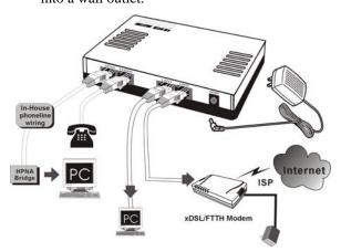
The figure above shows how to connect a cable modem to a home phoneline network. Follow the same steps to connect any Ethernet device such as a HUB or printer, to a home phoneline network.
